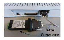
The DATA CONVERTER is connected directly to the RS232 serial line connector (SUB-D type 9 pins) on the back side of the printer.
