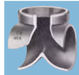
OPW-ES 464 Cast aluminum tee with female threads. Especially designed for handling jet fuel. Prevents high-velocity impingement on bottom of tank to reduce possibility of ignition of jet fuel. Available in 3" and 4".
